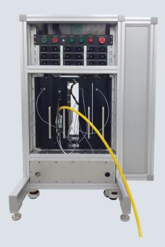
The LiComm OFL-CYR series is a 1080nm High Power Fiber Laser System with max. 3 Laser modules, a laser combiner, power supply, cooling distributor, and a control unit. The OFL-CYR series lasers offer high Beam quality and stable output power up to Mean Optical Power 3kW. Compact size (400 x 560 X 73 mm), combined with extremely low power consumption, allows the OFL-CYR series to be highly suitable for applications such as Welding, Cutting, Marking and more.
